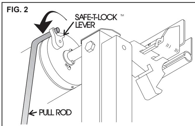
3. Insert hook of the pull rod through the loop of the pull strap. Pull the strap outward and completely extend the awning. The awning will stay positioned by itself. (FIG. 3)
