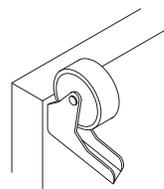
**Please note:** A slight "travel line" may appear where the door roller contacts the awning fabric. This is considered normal and does not affect the integrity of the awning.
