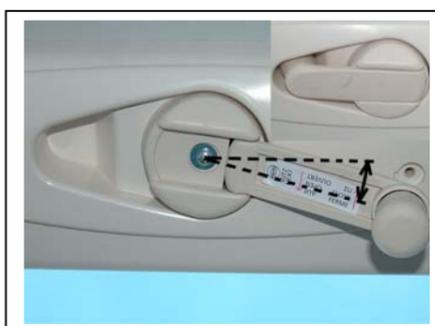
Turn the crank only until a resistance is noticeable during closing. Before throwing the crank a slight tension has to occur. Check the locking by lifting up the dome with the hand.
