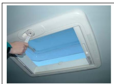
Turn the crank only until a resistance is noticeable during opening.
